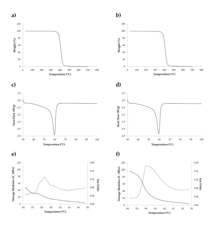
**Figure S1.** Thermogravimetric analysis of **(a)** 10%-PCL-ES scaffolds and **(b)** 15%-PCL-ES scaffolds. Differential scanning calorimetry of **(c)** 10%-PCL-ES scaffolds and **(d)** 15%-PCL-ES scaffolds. Dynamic mechanical analysis of **(e)** 10%-PCL-ES scaffolds and **(f)** 15%-PCL-ES scaffolds.
