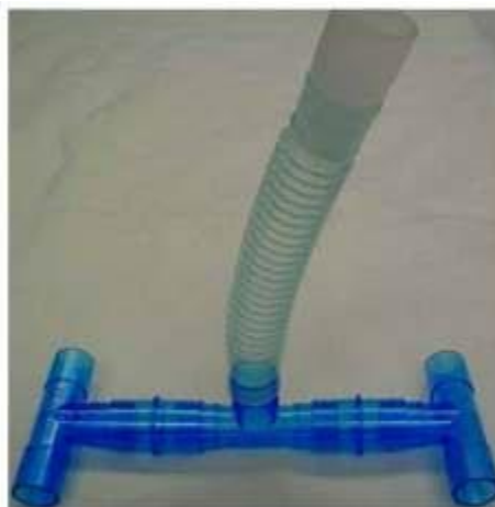
Figure 2. Flow splitter configuration of three T-tubes with connection adapters (shown here with trimmed section of ventilator tubing).
