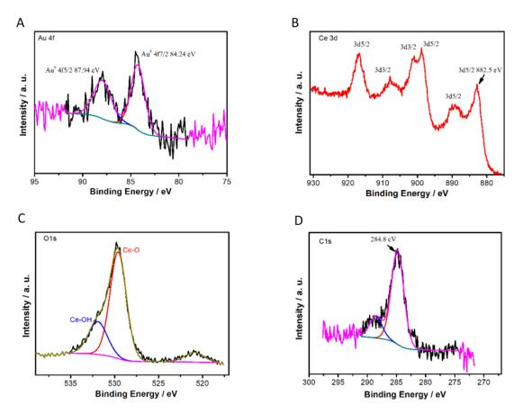
**Figure 4.** Experimental high resolution XPS peaks, best deconvolutions and assignments of Au 4f (**A**), Ce 3d (**B**), O1s (**C**) regions for a sample of 0.82% Au/CeO<sub>2</sub> and C1s (**D**) XPS spectra used as reference.
