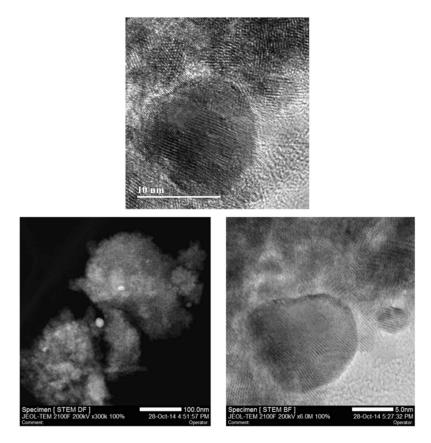
**Figure 1.** Representative HR-TEM (**Top**), dark Field (**Bottom**, **Left**) and bright Field (**Bottom**, **Right**) HR-STEM images of the 0.82% Au/CeO<sub>2</sub> catalyst. The high-resolution image allows one to distinguish the crystal planes corresponding to Au particles. Au element is well distributed in the particles, as observed in the bright field image.
