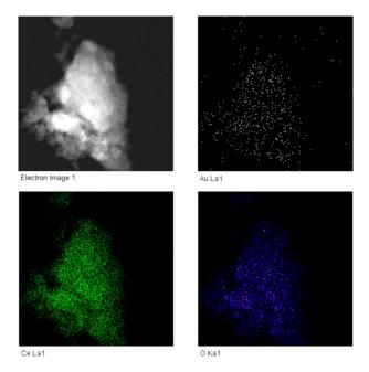
**Figure 2.** Dark field scanning electron microscopy of 0.82% AuCeO<sub>2</sub> catalyst and EDX elemental mapping of gold, cerium and oxygen demonstrating that these elements are evenly distributed in the particle.
